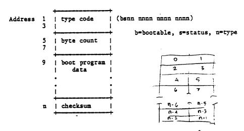
The type code is a 16 bit female byte sex number (most significant byte first) stored in the first two bytes of the ROM. If the first bit is a 1 (see above), the device claims to be bootable. If the device's status should be checked at boot time, its status bit (the second bit) is a 1. The other 14 bits are the identification number which identifies the card.
